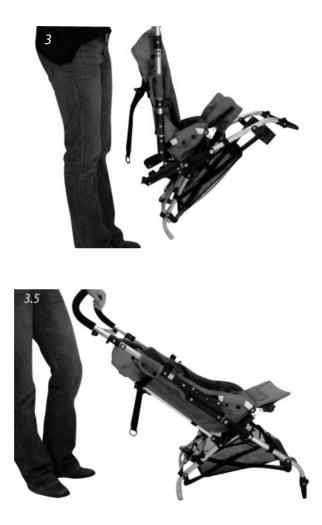
Using your foot, engage the rear frame support bars (4).
